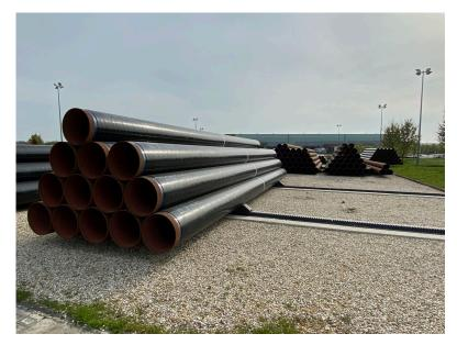
Pipe Stop enables a safe working environment and prevents employees to work between the pipes during the handling processes.
