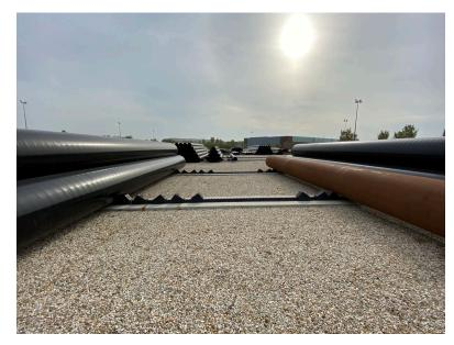
Besides being able to prevent coating damage and enable spacing between each pipe, Pipe Stop offers the advantage of supporting sideways on two surfaces, which reduces the ovality.
