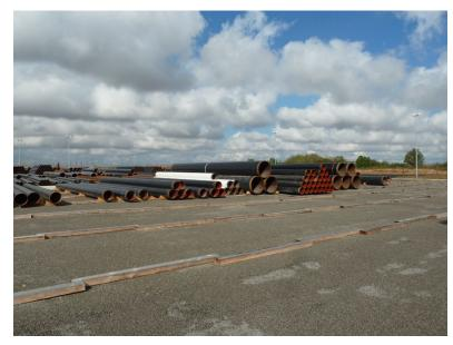
Wood used as support for the pipes. In some cases the coating of the pipes would be damage and dangerous situations would be created.
