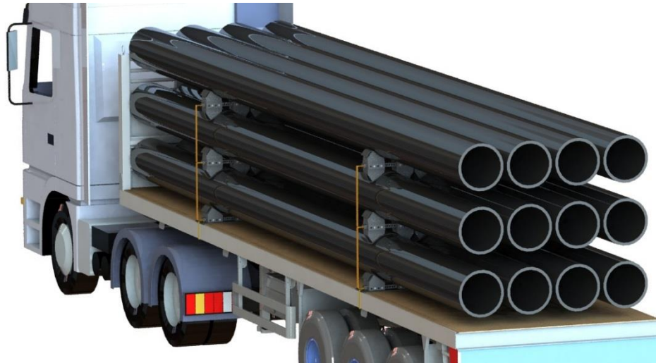
Figure 21. Place remaining layers
