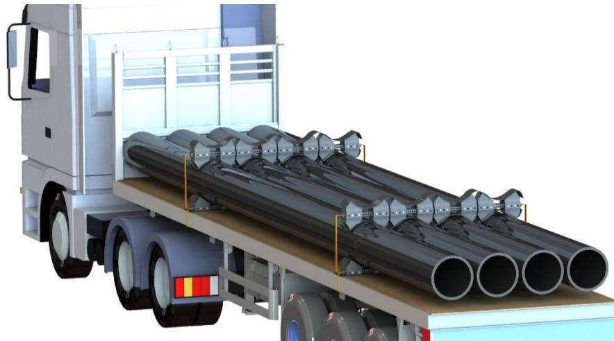
Figure 20. Place Anti-skid on the mid-section (Truck only)
