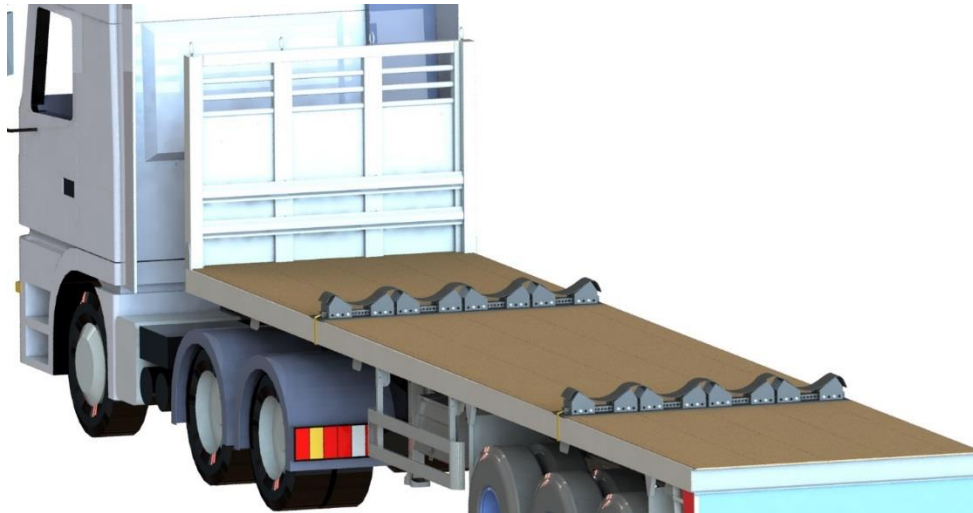
Figure 15. Place Anti-Skid on top of the blocks (truck only)
