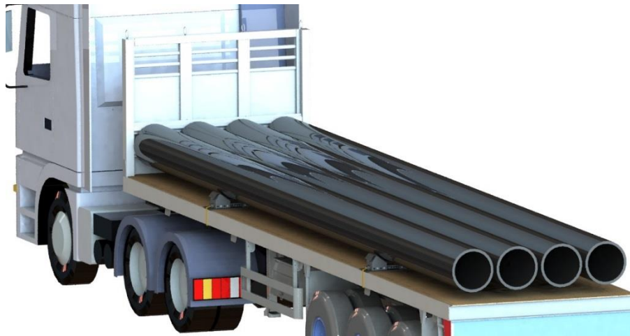
Figure 16. Place pipes on the bottom blocks
