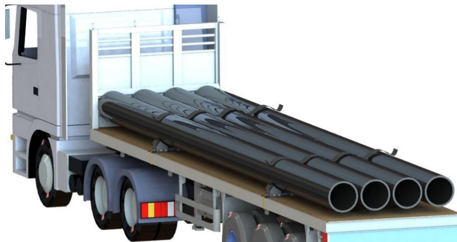
Figure 17. Place Anti-skid on the bottom layer
