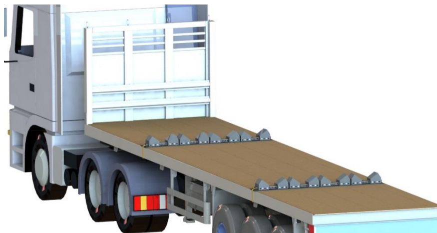
Figure 14. Lock the blocks with a pin and place profile-to-trailer connectors
