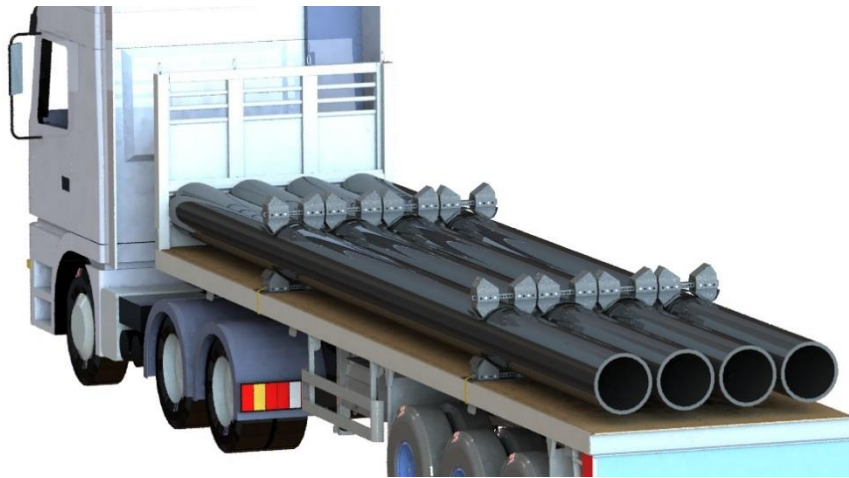
Figure 18. Place the mid-section with blocks on top of the bottom layer
