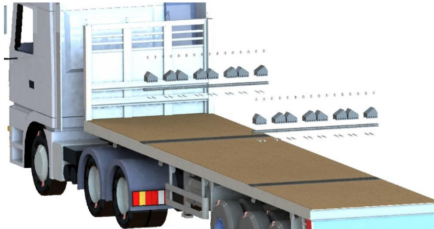
Figure 11. Start set-up with Anti-skid in place (trucks only)
