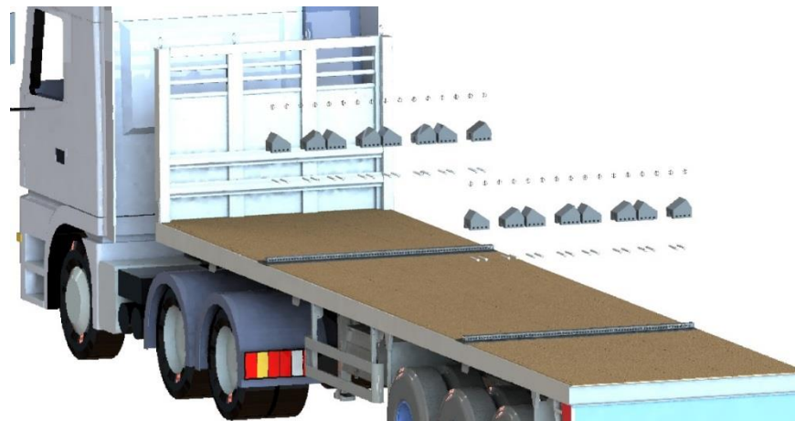
Figure 12. Fasten profile to trailer
