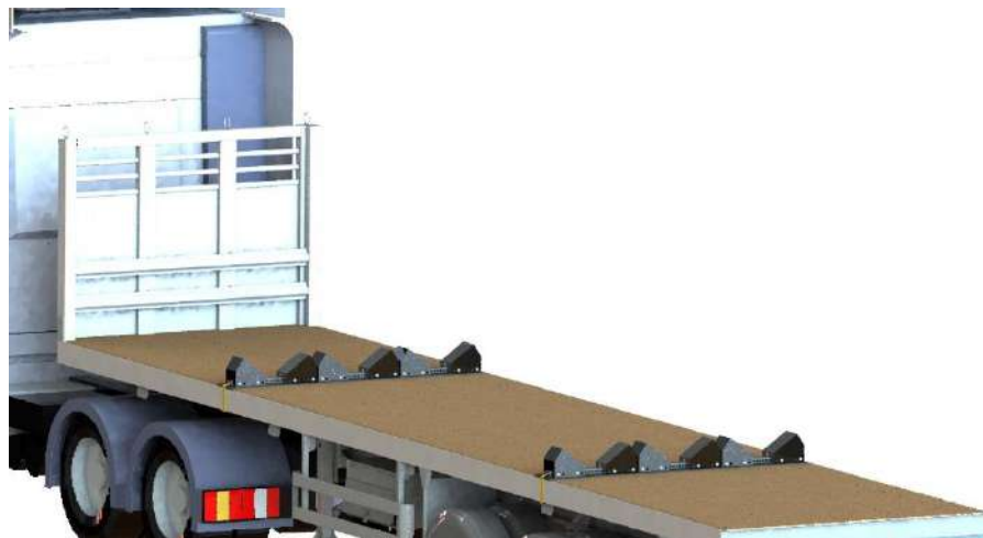
Figure 14. Lock the blocks with a pin and place profile-to-trailer connectors
