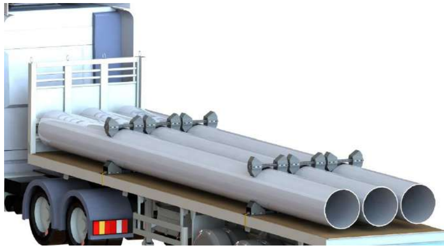
Figure 18. Place the mid-section with blocks on top of the bottom layer
