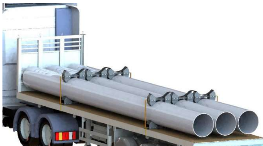
Figure 20. Place Anti-skid on the mid-section (Truck only)
