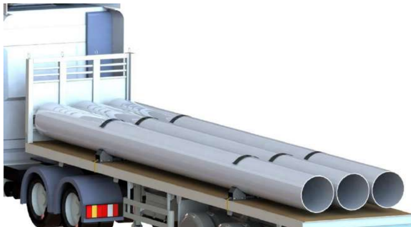
Figure 17. Place Anti-skid on the bottom layer (Trucks only)
