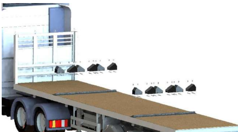
Figure 12. Fasten profile to trailer
