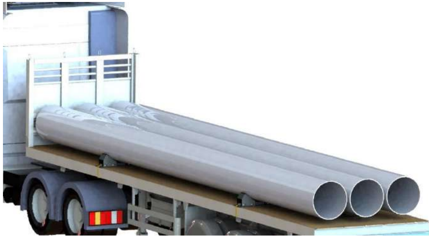
Figure 16. Place pipes on the bottom blocks
