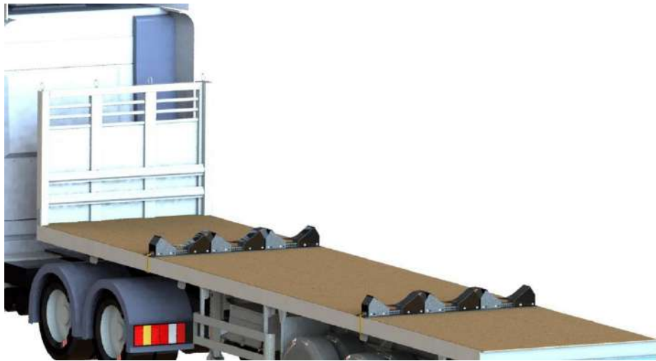
Figure 15. Place Anti-Skid on top of the blocks (truck only)
