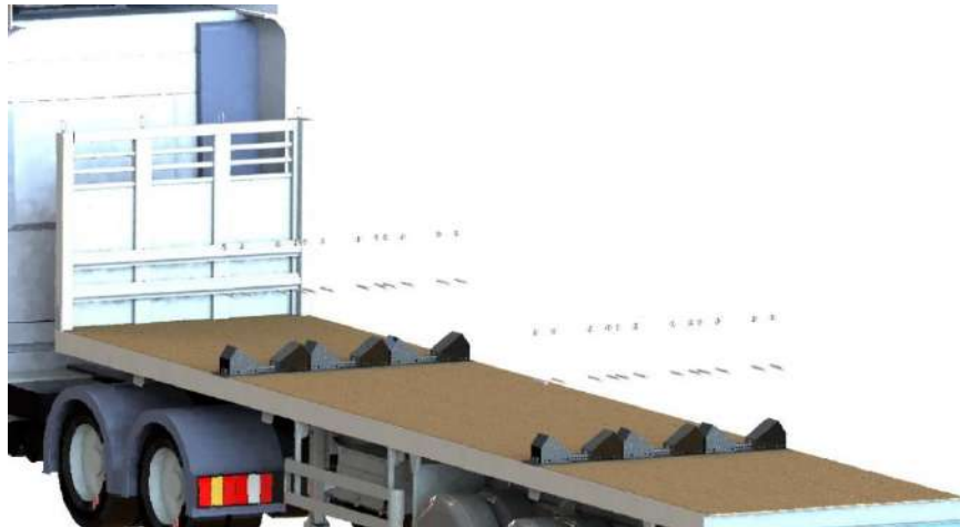
Figure 13. Place block on profile
