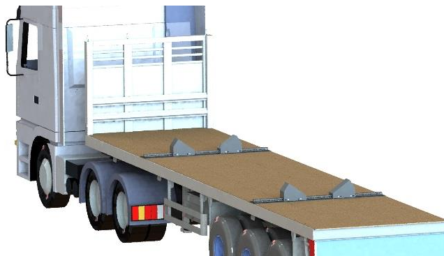
Figure 10. Lock the blocks with a pin and place profile-to-trailer connectors
