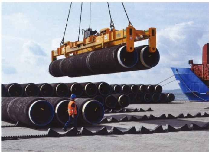
Figure 2. Heavyweight concrete coated pipes being stored on a new storage system.
