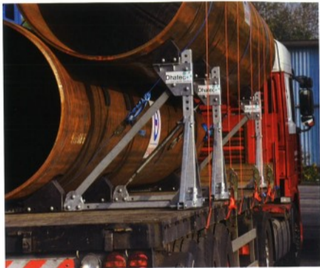
Figure 9. Two 56 in. pipes on Pipe Raiser.
