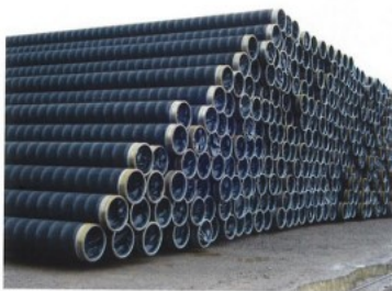
Figure 5. Bevel protector and sheets, economically attractive for short-term storage.
