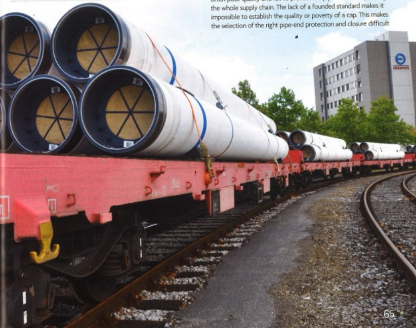
Figure 1. Dhatec plug with breathable membrane. These types of plugs withstand handling and transportation vibrations perfectly.
